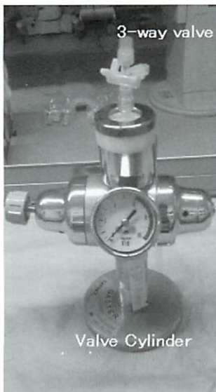
Fig. 1 The author flush CO 2 every 3 minutes by plastic syringe with 3-way valve.
